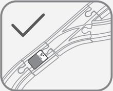
Paste the turn right sticker on the straight track that connects with the Y track to make the train turn right at the Y track.
